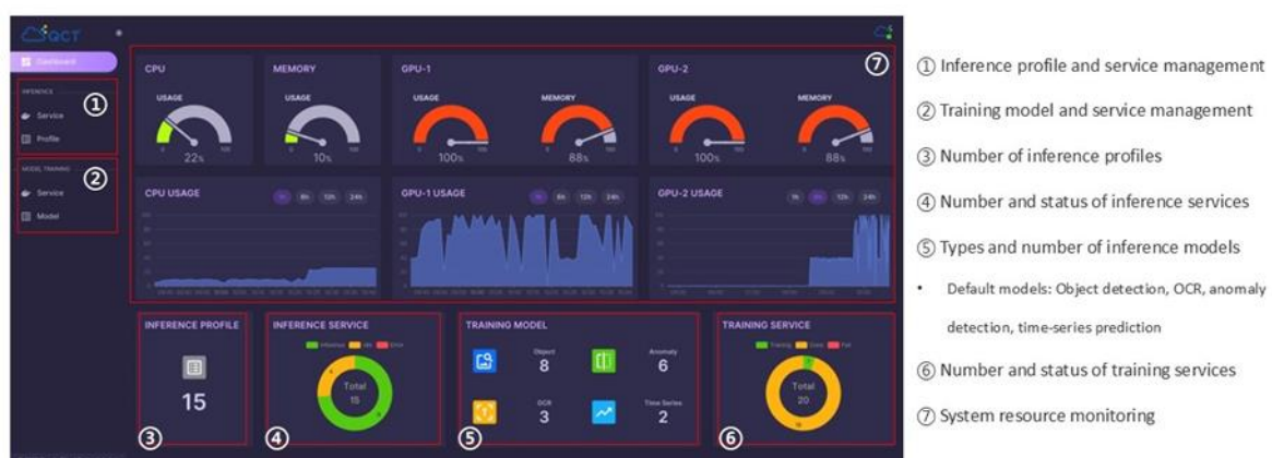
Figure 8: The QCT 5G x AI Dev. Kit's GUI for AI training and inference processes
